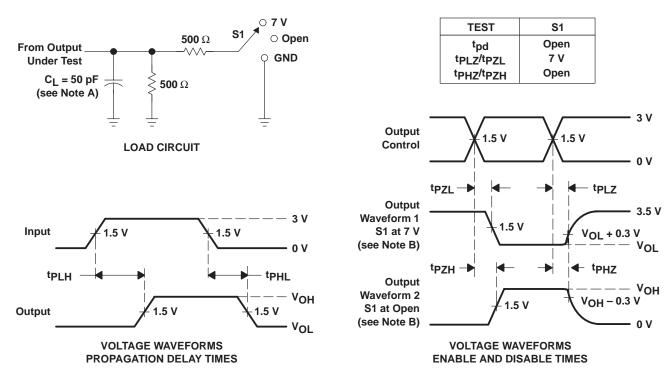
NOTES: A. C<sub>L</sub> includes probe and jig capacitance.
